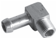
080955 Std pkg 10 A Screw terminal 1/8-27 NPTF. For 8 mm. hose I.D.
