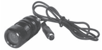
160610 Colour camera (Bumper fit, Biuld-in) • Aluminium w/original anodised finish and anti-fog glass. • 30 mm. (O.D.) x 65 mm. (L), 200g • Wide view angle, 110° diagonal. • Sensitivity < 1 LUX. • W/ mirror function (on camera) • Protection degree: IP 68. • Connection: 6pin Mini DIN. Standard camera in following kits: Cargo 160662, -664.
