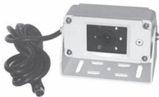
160609 Colour camera cased in waterproof aluminium housing for protection against foul weather and shock/vibration. • Wide view angle, 150° diagonal. • Infrared LED's for night vision. • Built-in microphone. • Connection: 6pin Mini DIN. • Protection degree: IP67. Standard camera in following kits: Cargo 160602, -604, -605, -606 and -775.
