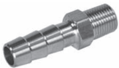
080955 Std pkg 10 A Screw terminal 1/8-27 NPTF. For 8 mm. hose I.D.
